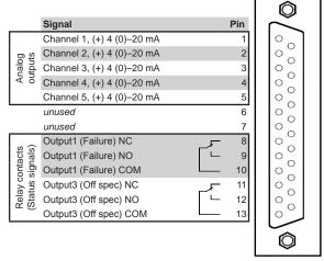
Fig. 4-13: Socket X1 - Analog & Digital Outputs 1-4
